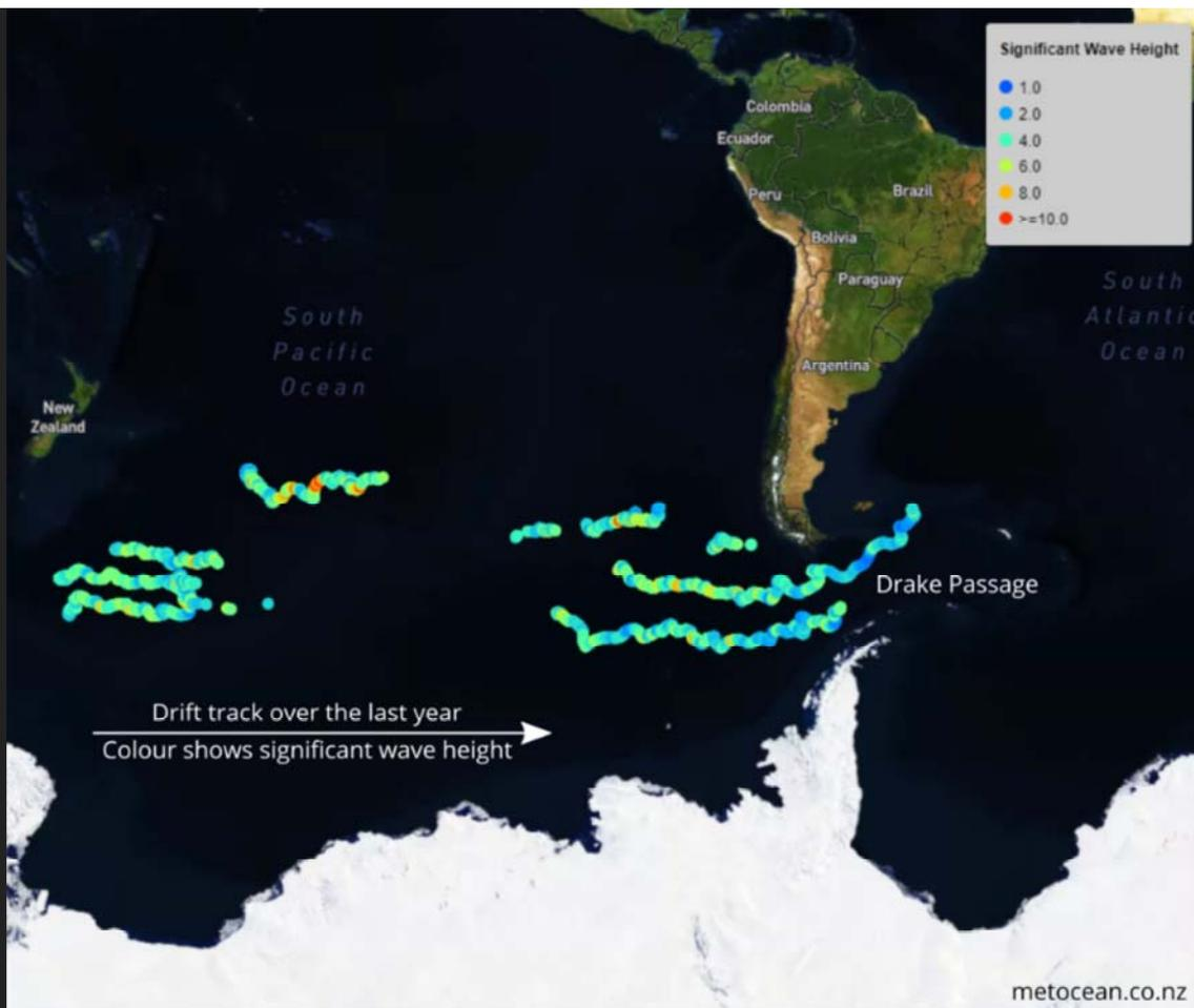
The Spotter's drift track and significant wave height measured over the last year.
